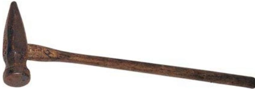
This rivet hammer was used to knock red hot rivets into steel plates. Riveting was an important part of building the Titanic. Riveting squads in the Harland & Wolff shipyard were usually three men and one or two young boys aged 14 or older. A boy heated the rivets in a furnace to a temperature of around 650 degrees Celsius. Then a boy, called a 'Heater' or 'Rivet Catcher', would hold it in tongs and run or climb to where it was needed before it cooled off.
